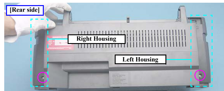
Figure 4-16. Removing the Right/Left Housings (1)
