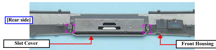
Figure 4-39. Removing the Slot Cover
