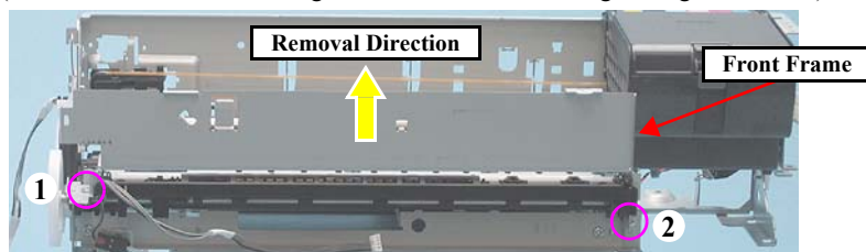
Figure 4-129. Removing the Front Frame
