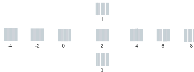
Figure 5-4. Bi-D adjustment Pattern Printing
