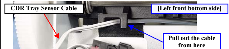
Figure 4-161. Routing the CDR Tray Sensor Cable
