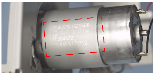
Figure 4-125. Reinstalling the CR Motor
