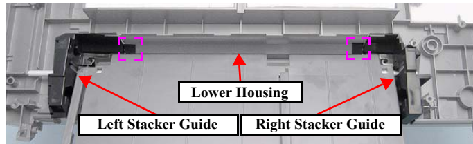
Figure 4-114. Reinstalling the Stacker Assy
